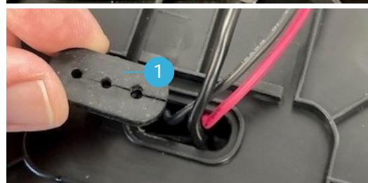
Carefully remove the rubber gasket (1) with a screwdriver.
