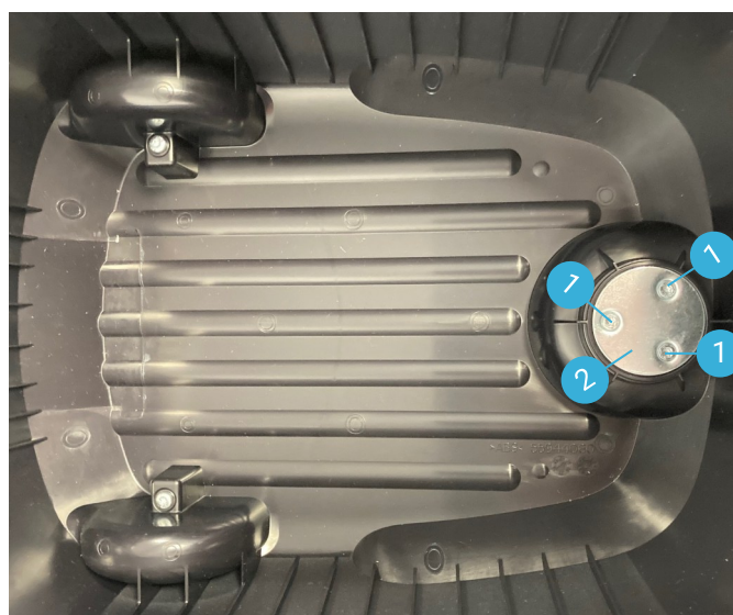
Remove the three screws (1) torx 20 for the castor wheel. Castor wheel and mounting plate (2) can now be removed.
