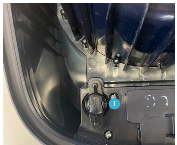
Vacuum valve (1). Valve ensures cooling for the turbine if the bendend/hose/bag is blocked
