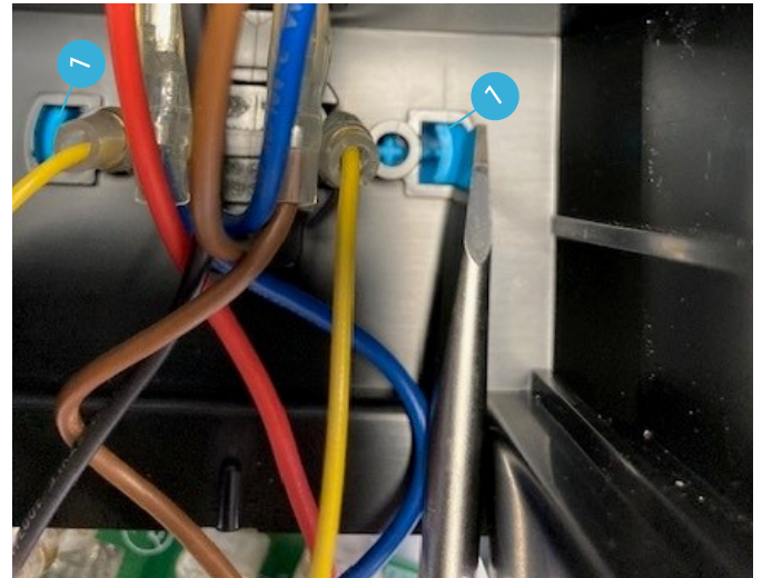
Release the two snaps (1) with a screwdriver and pull out the eco mode button (1). Single mode machines have no eco mode button
