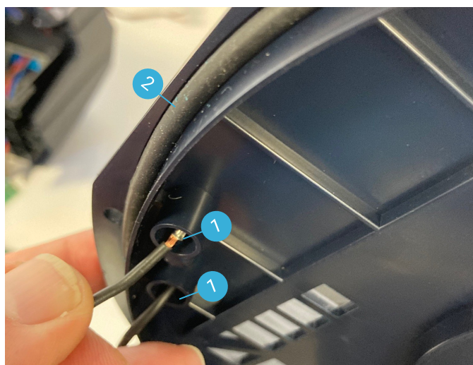
Route the two wires to the turbine through the two holes (1). Make sure the foam gasket (2) is correctly positioned around the filter plate.
