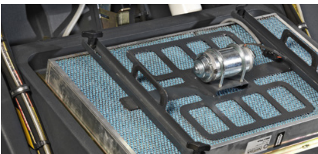
Filters Paper filter: Works well in dry, high dust conditions Polyester: Excellent in moist applications, can be washed, dried and re-used
